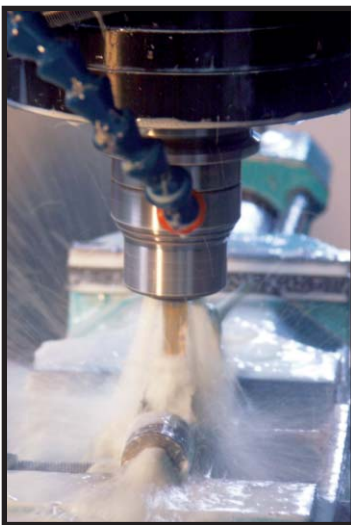
Standard Collet – coolant is delivered through the slots.
