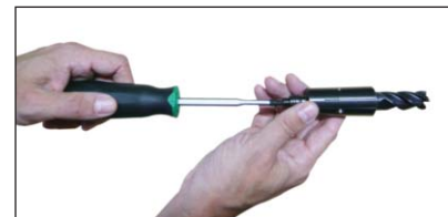
3 – Using our pre-set torque driver, tighten the collet depth stop against the back of the end mill.
