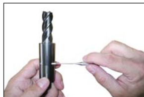
2 – Use the insertion tool to push the locking pin into place.
