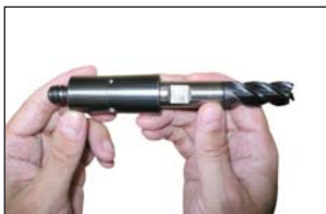
1 – Insert the end mill into the collet, making sure the Weldon flat is aligned with the cross-drilled hole as shown.
